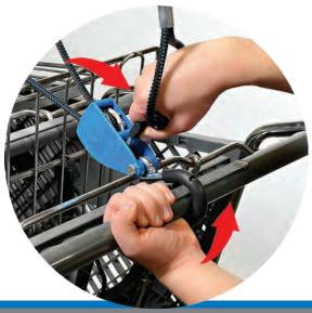
Easing tension on the ratchet release lever as illustrated will extend it's useful life!
